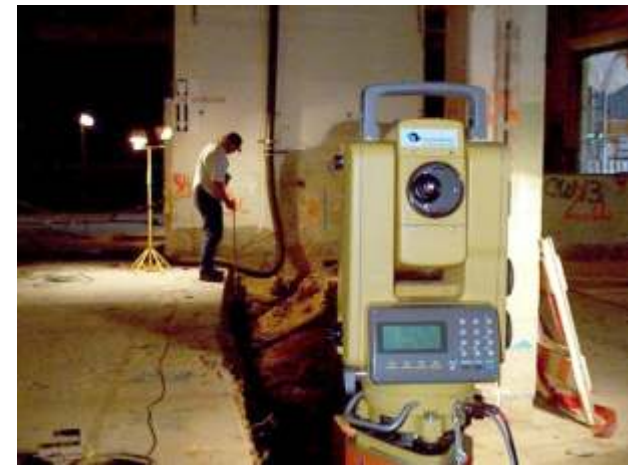
We use LARADS for indoor surveys or in outdoor areas where GPS signal is unreliable.
